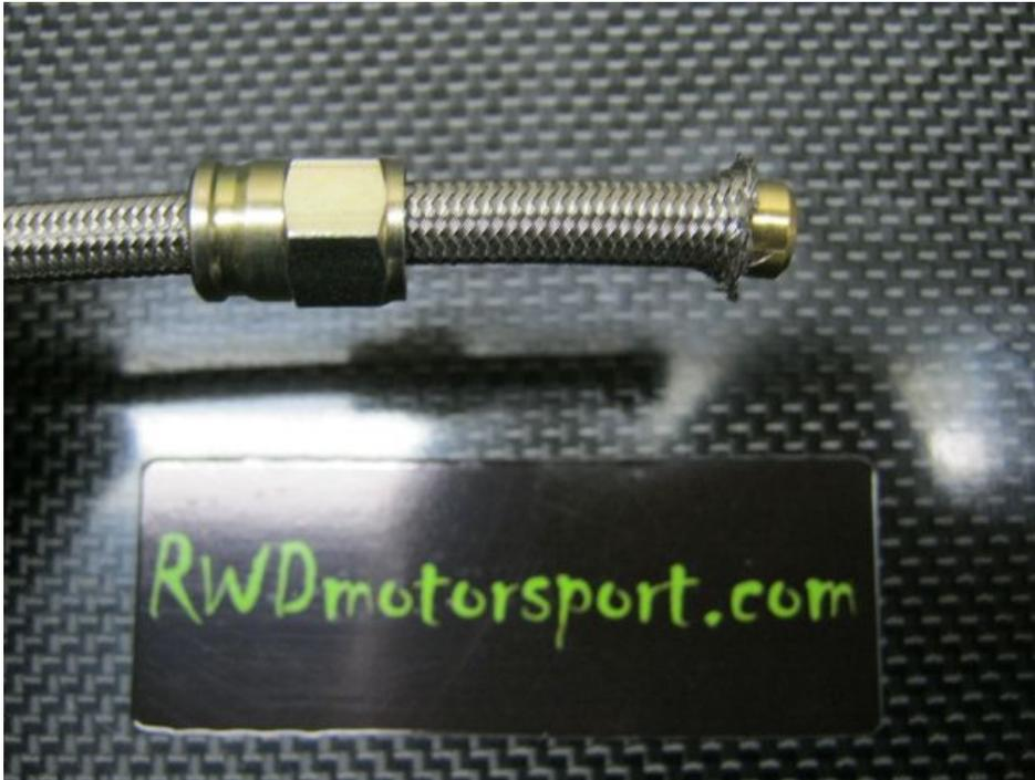
Push on the brass olive taking care not to get any strands of the braiding between the olive and PTFE inner hose.
