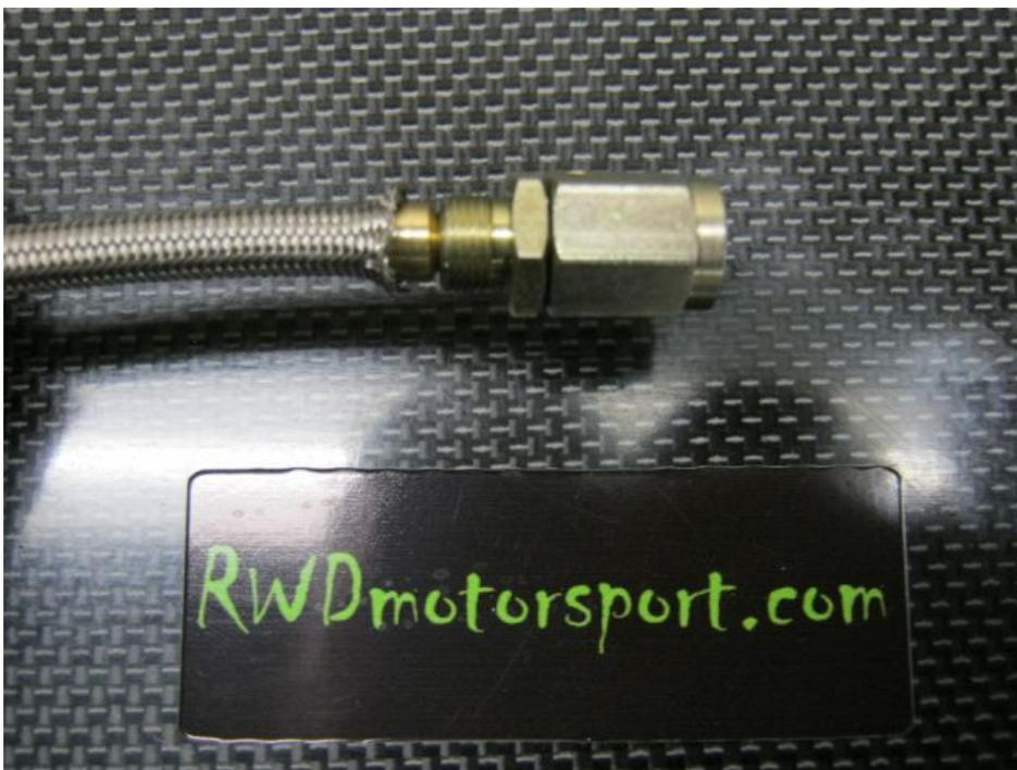
Push the small tube on the fitting into the end of the hose, then slide the nut over the flared out braiding keeping the fitting pushed up against the brass olive. Screw the nut onto the fitting (if the nut doesn't start on the thread there may be a stray bit of braiding needing trimming). Next tighten using 2 spanners leaving approx 1mm gap between the nut and fitting.
