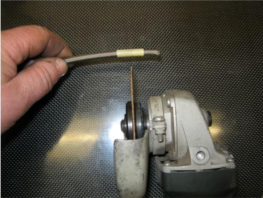
Wrap a couple of turns of masking tape tightly around where the hose needs cutting.
